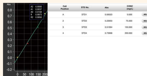
Example of a calibration curve in the concentration measurement mode
