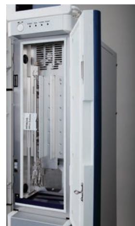
A view of column oven accommodating columns
